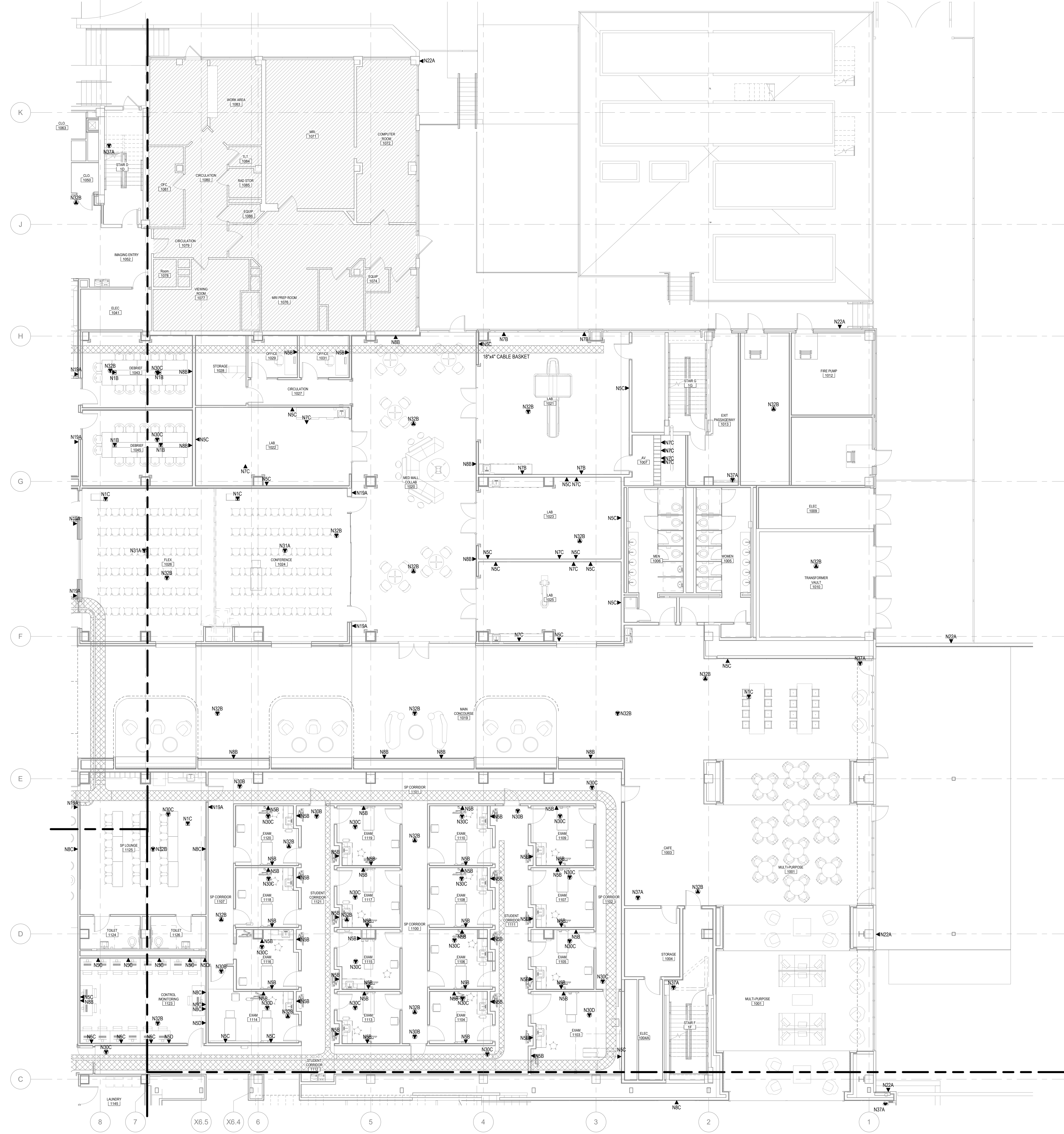
TELECOMMUNICATIONS FIRST FLOOR AREA C PLAN 1/8" = 1'-0"
